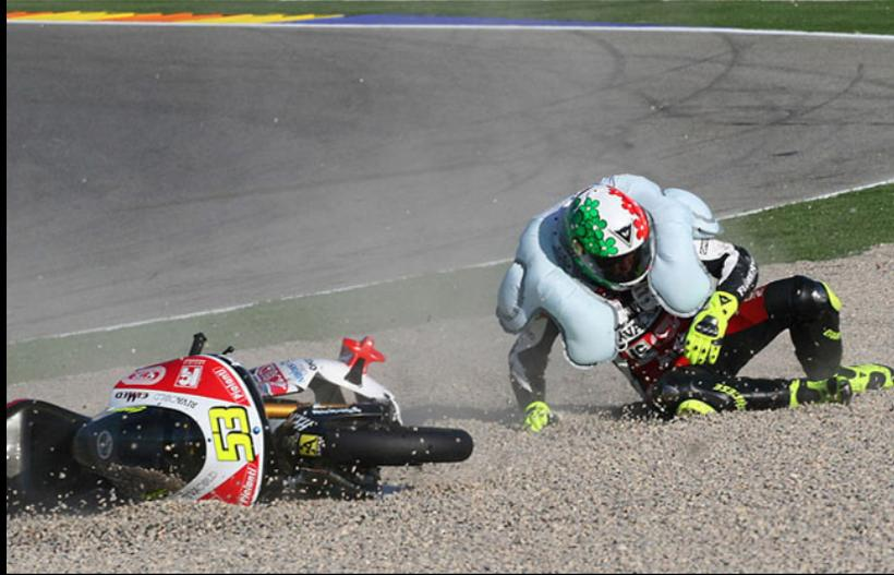
It's a suit with a self-contained deployable airbag when subjected to impact. The manufacturer believes it has significant potential to decrease injury after an impact on a motorcycle.
